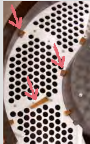
Polyurethane wedges allow quick screen fastening and ex-change of screens.
