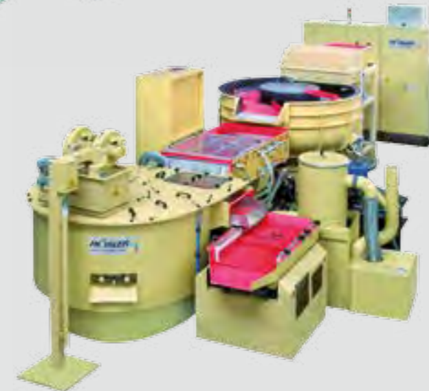
Parts loading: Vibratory feed hopper. Vibratory washer for finished parts; drying with vibratory dryer linked with special vibratory screening unit to remove residual drying media from the finished parts
