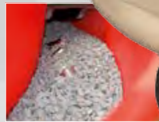
Optimum immersion of parts into media mass; protection against parts nicking each other on the channel incline
