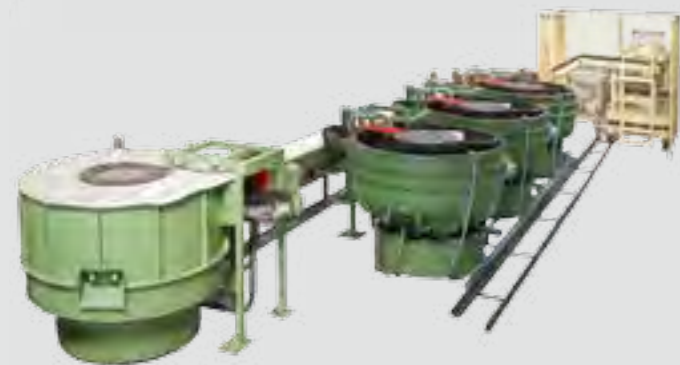
Parts loading: Load system movable on rails with integrated vibratory feed hopper Conveyor belt for collecting finished parts and transferring them to a vibratory dryer
