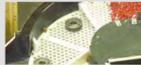
Separation screens with built-in tumbling steps Removes media from cup shaped parts
