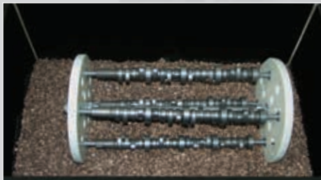
Delicate parts are mounted onto a fixture. This allows the processing of multiple parts without any danger of nicking.
