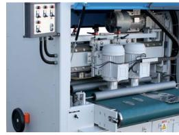
Height adjustment by handwheel or motorized (option)
